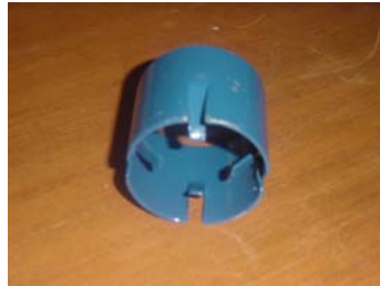
Figure 3. AMDP manual corn sheller.
